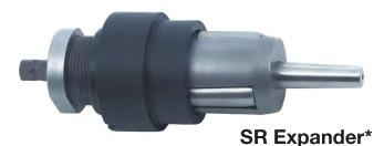
The "SR" Short Reach Expanders incorporate a rapid taper on the mandrel that allows full expansion of a tube with minimum travel of the mandrel. The mandrel is retained at the rear of the expander to shorten the mandrel length which allows use near sharp tube bends. These expanders are made to order so application details must be provided ahead of time.
